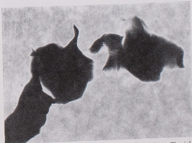
Phot. 2. Electron micrograph of montmorillonite from Chmielnik show mainly thick, irregular, sharp-edged particles. Magn. \times 21,000
